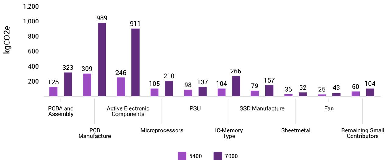
**Figure 6 Manufacturing and assembly impact breakdown (GWP 100 emissions from manufacture)**
